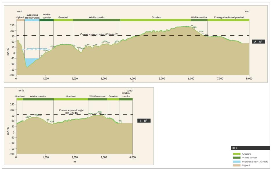
Figure 2: Indicative Final Rehabilitated Landform Cross-Sections
